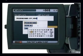
The P2 cam records each recording as a clip (file) and automatically attaches a thumbnail image and file information to it. To preview a clip on the LCD monitor or to check clip data, simply choose the clip you want from the list of thumbnails. It also supports metadata input using a new software keyboard.
